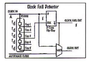
A multitap delay must be used because the time from the first rising edge of the clock to the sampling point  $(t_D)$  is slightly more than one full clock period  $(t_{WH} + t_{WL})$ . Since the "minimum input pulse width" specification restricts us to one-half period delay maximum, the simple solution is to break down the delay into three smaller increments, such as is provided in a multitap device.
