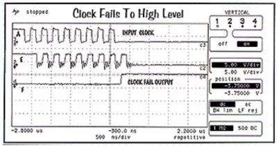
If the clock fails high, an inverter on the CLK input of the flip-flop and the use of the Q rather than the  $Q\setminus$  output can be used instead. The resulting waveforms can be seen in the diagram.
